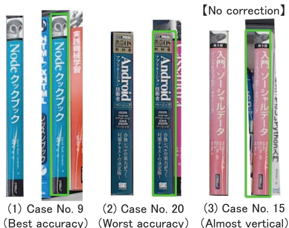
Figure 22: Influence analysis of gesture indication error on template-matching accuracy
