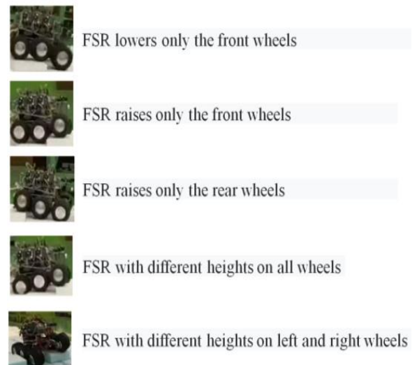
Figure 13: Driving of FSR with high grounding capacity.
