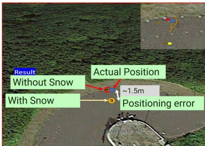
Figure 5: Positioning error caused by Snow accumulation
