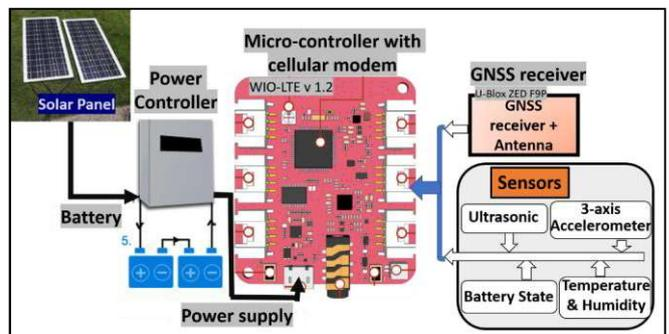
Figure 8: Block diagram of the base station
