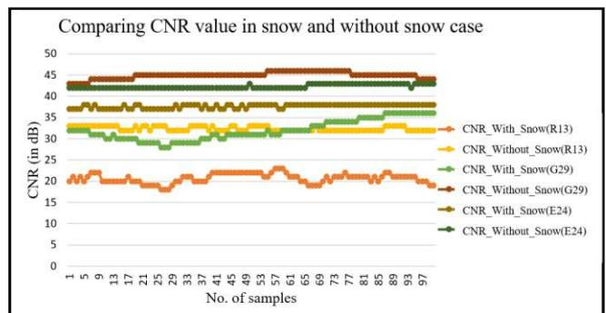
Figure 4: Snow effects in Carrier to Noise Ratio
