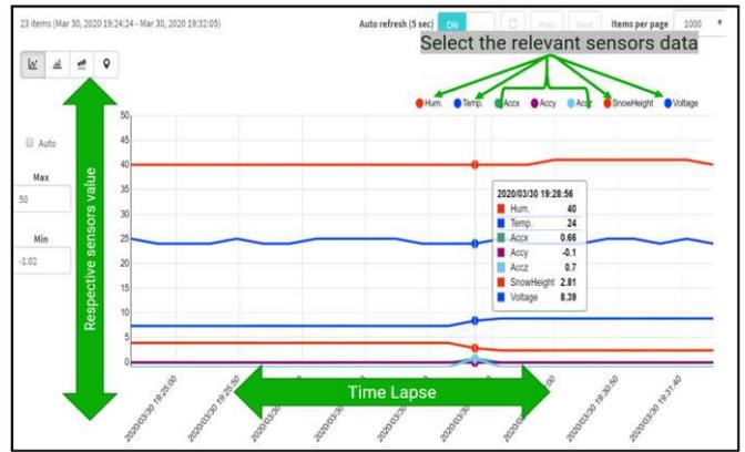
Figure 14: Graphical view of sensors data on webpage
