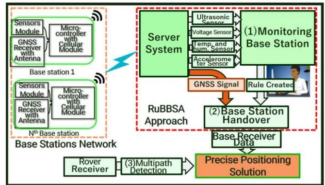
Figure 6: System architecture
