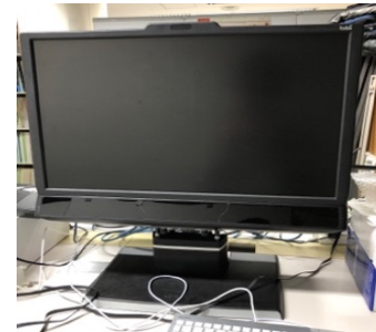
Figure 2: Measurement equipment (Tobii Pro Tx-300)
