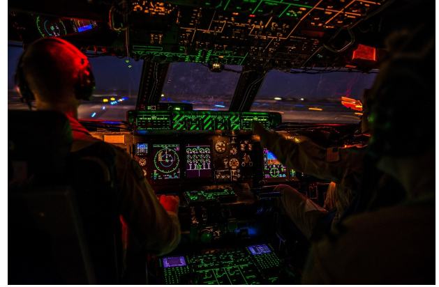
Figure 15: Cockpit of an airliner. Not all visual displays lie in the visual focus. Some may even be occluded by the pilot or the copilot.
