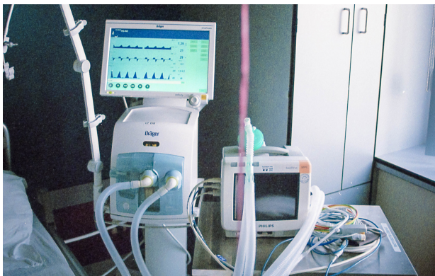
Figure 20: User interface for monitoring a patient's vital functions. A monitor is combined with an auditory display to serve as a multi-modal user interface.
