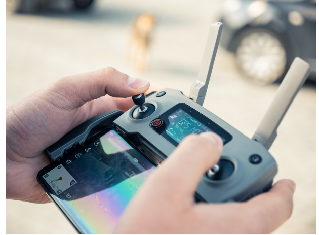
Figure 9: Typical drone remote. A visual UI shows the camera view overlain by graphics that indicate spatial relations, like drone coordinate and orientation, and distance and direction of obstacles.
