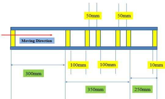
Figure 13: Schematic of the testing board with an uneven surface
