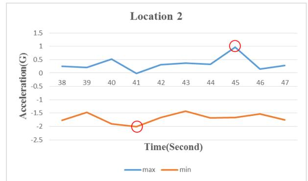
Figure 22: MAX/MIN accelerations at the second uneven site along the outdoor route
