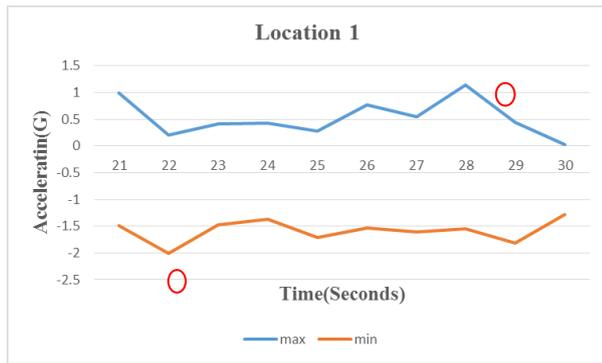
Figure 21: MAX/MIN accelerations at the first uneven site along the outdoor route
