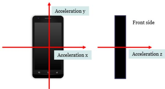
Figure 7: Acceleration components of the smartphone
