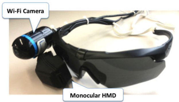
Figure 3: Monocular HMD and Wi-Fi camera
