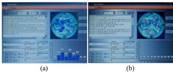
Figure 27: GPS signal conditions. (a) Outside of a tunnel;, (b) Inside of a tunnel
