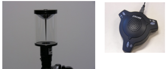
Figure 2: Devices used for recording daily informal communication: Omnidirectional camera (left) and a conference microphone (right).
