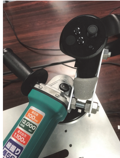
Figure 2: For the repulsion experience, Oculus touch is attached to the upper right part of the actual grinder.
