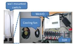
Figure 6: Devices used to control fluorescent lights
