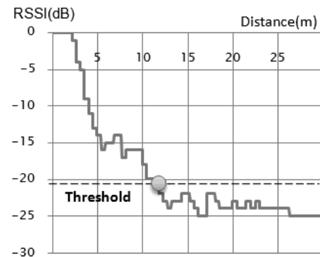
Figure 12: Example of change of RSSI with distance
